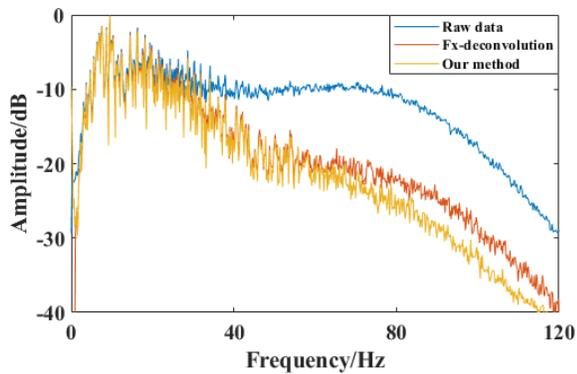
Fig. 5. Multichannel average amplitude spectrum of raw data and denoised data.
