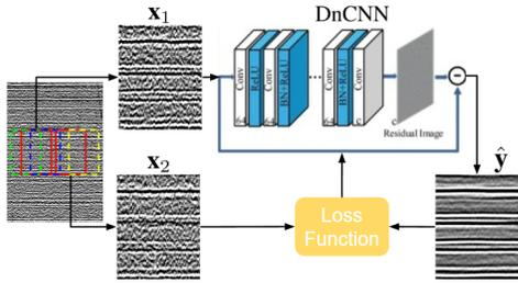
Fig. 1. Schematic of the proposed denoising framework
