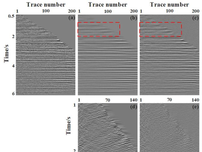
Fig. 4. Denoising comparisons of field seismic data. Denoised results using (b) our method and (c) f-x deconvolution. Removed noise using (d) our method and (e) f-x deconvolution of the enlarged area of the red boxes in (b) and (c).
