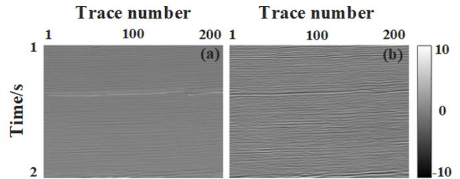
Fig. 7. The stack section of noise removed by (a) our method and (b) f-x deconvolution.
