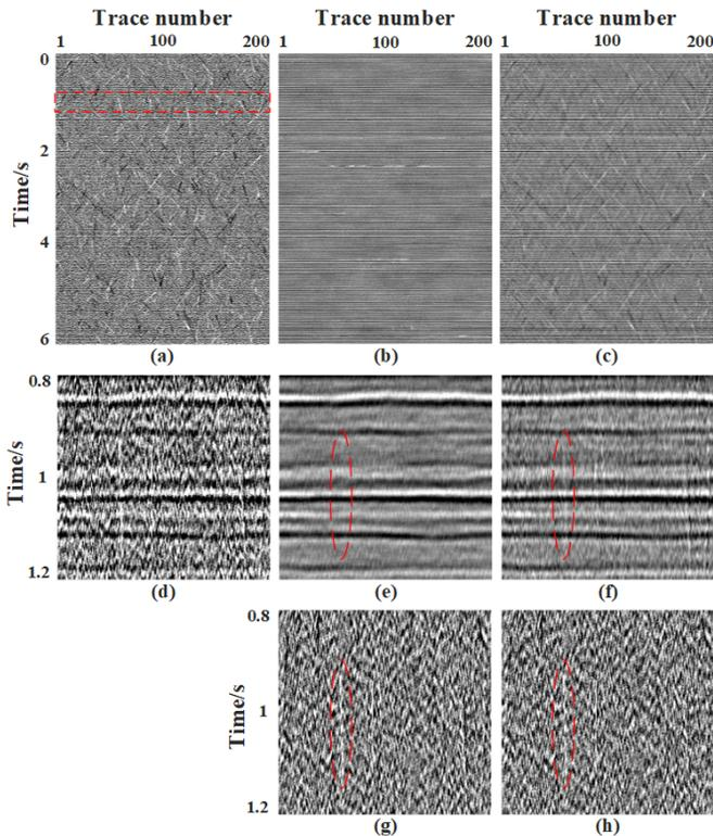
Fig. 3. Denoising comparisons of synthetic seismic data with dense coherent noise. (a) Raw data. Denoised results using (b) our method and (c) f-x deconvolution. (d) Enlarged raw data. Enlarged denoised results using (e) our method and (f) f-x deconvolution. Removed noise using (g) our method and (h) f-x deconvolution.
