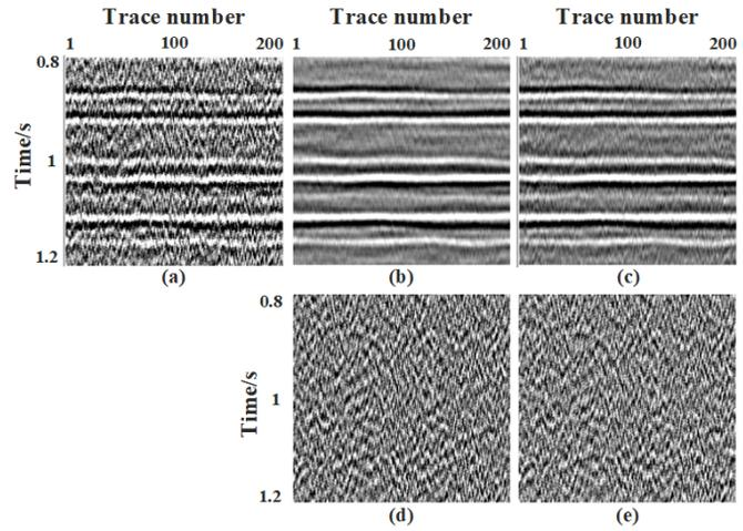
Fig. 2. Denoising comparisons of an enlarged area. Denoised results using (b) our method and (c) f-x deconvolution. Removed noise using (d) our method and (e) f-x deconvolution.
