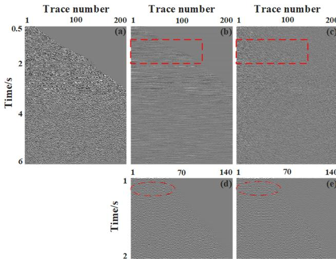
Fig. 6. The 50 Hz high-pass filter results of (a) raw data and denoised data using (b) our method and (c) f-x deconvolution. The 50 Hz high-pass filter results of removed noise using (d) our method and (e) f-x deconvolution of the enlarged area of the red boxes in (b) and (c).
